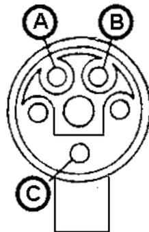
Use a piece of wire to bridge test port B and C
