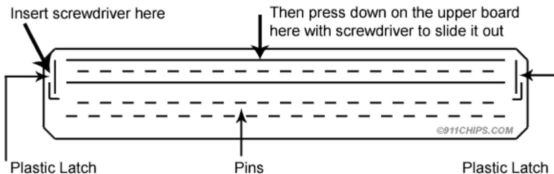
***Disassembling the DME connector plug***
